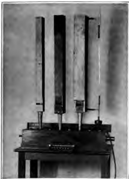
FIG. 133. Organ pipes for demonstrating the influence of the walls on the tone.
